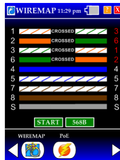
Example - Crossed 12-36 shielded cable
